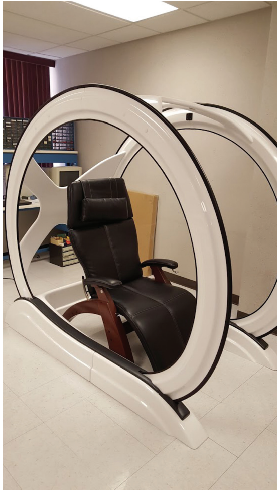
Fig. 1. The Resonator® device. The simplified Helmholtz coil system is 7 feet in diameter with 3.5 feet of separation. The system is designed to create a homogenous, isotropic magnetic field from 1 to 99 pT with a frequency range of 0.01 Hz to 50 Hz.
